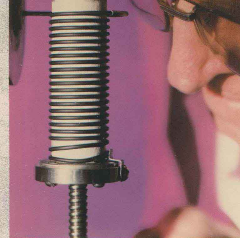
Fabricating a superconducting coil is made easier with Argonne National Laboratory's new extrusion process, shown here producing a 3-cm-diameter coil of "1-2-3" wire.
