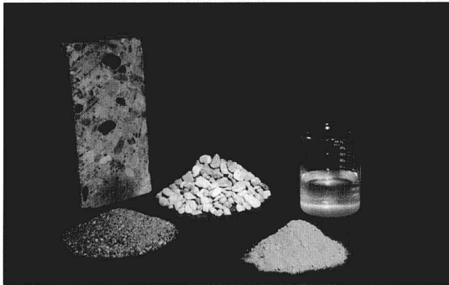
Fig. 1-1. Concrete components: cement, water, fine aggregate and coarse aggregate, are combined to form concrete. (55361)
