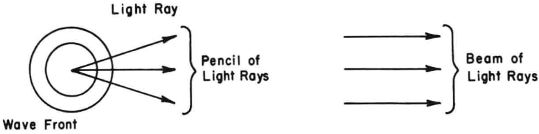
Fig. 1-1. A light ray is a line drawn perpendicular to a wave front of light emitted from a source. Parallel pencils of light rays form a beam.
