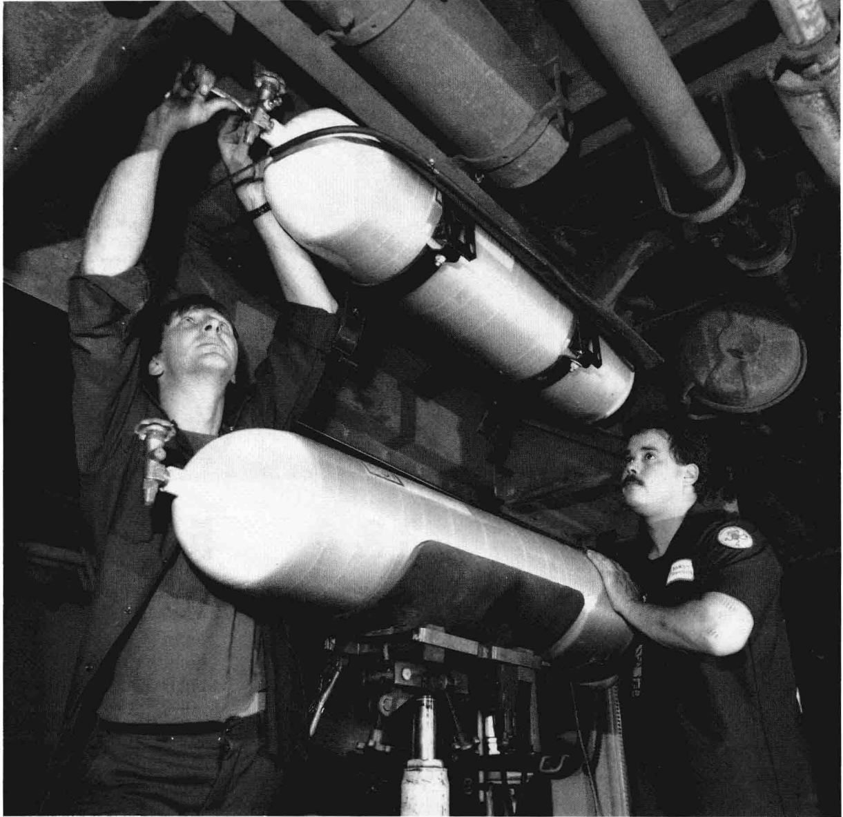
FIGURE 1.3. In vans and pickup trucks, natural gas cylinders can be installed under the vehicle. In cars, they can be placed in trunks. In either case, the tanks are put into a position where they are well-protected from rupturing in the event of a collision. The three cylinders shown in this photograph were installed in a UPS van and supply that vehicle with the equivalent of 15 gallons of gasoline. (Courtesy of Brooklyn Union Gas Company)
