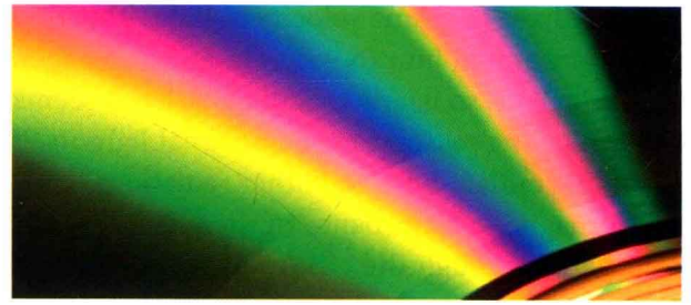
FIGURE 2.4. Diffraction of light from the surface of a compact disc. The pitch of the data tracks is 1.6\ \mu\text{m} , and each angle of reflection selects a specific spectral color.
