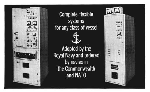
■ Precise frequency setting and positive stability allows full advantage to be taken of SSB which provides the most reliable communications under difficult conditions of propagation or interference ■ Continuous frequency coverage from 240 Kc/s to 24 Mc/s ■ Covers all types of signalling ■ Broadband amplifier and synthesizer system provides simplest operation and almost eliminates tuning ■ Aerials can be sited for maximum radiating efficiency.
