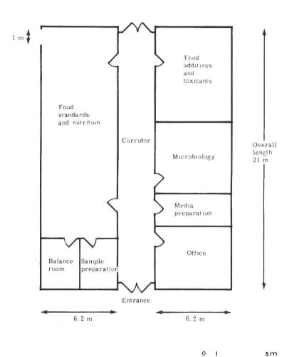
Figure 3.1 A Minimum Sized Food Control Laboratory
