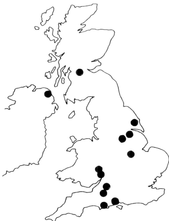
Fig. 5. Locations of existing deep seismic reflection data sets on land in the United Kingdom between 1979 and 1982 (after Whittaker and Chadwick, 1983). Profiles range in length from 1.5 to 30 km with two-way travel times of 6 s or greater.
