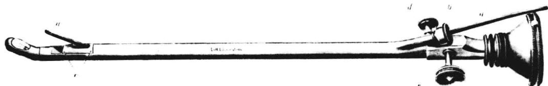
Figure 1.6 Nitze's cystoscope—later model with electric bulb illumination shown with ureteral probe inserted through channel. (Reproduced with permission, courtesy of National Library of Medicine, Bethesda, Maryland.)
