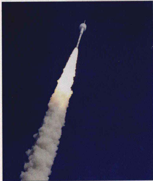
A bow shock forms around the Ares I-X traveling at supersonic speed. The rocket produces 2.96 million lb of thrust at liftoff and goes supersonic in 39 sec. Liftoff occurred on October 28.
