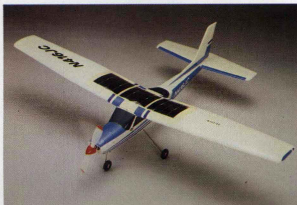
(6) Example of an application of amorphous Si solar cells formed on a flexible film (photograph supplied by Teijin).
