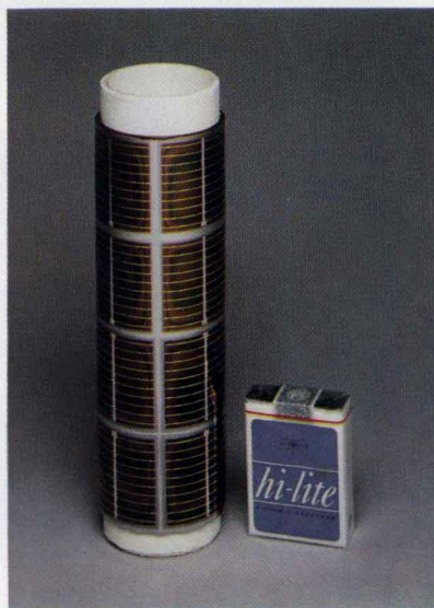
(5) Amorphous Si solar cells formed on a flexible film (photograph supplied by Teijin).
