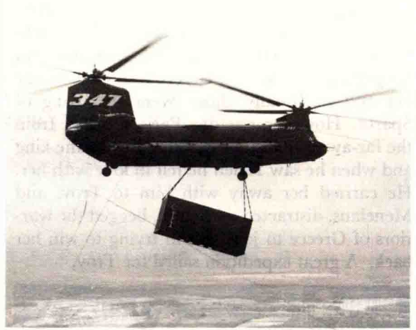
Left: the Cierva autogyro of 1928 was the pioneer of rotary wing flight. Right: The Boeing CH-47 has two four-bladed rotors. In this experimental model, known as the 347, a controllable, tilting wing was added to improve the helicopter's manoeuvrability.
