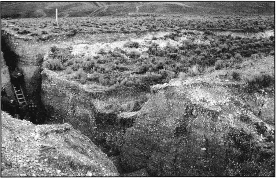
The rupture trace of the 1983 M_s 7.3 Borah Peak, Idaho earthquake (Lost River fault zone) approximately 50 m north of the Doublesprings Pass Road, is dominated by a 15-m-wide graben. One year after the rupture, a 3-4-m-deep, 45-m-long trench (left and lower center) was excavated across the fault trace to identify and characterize paleoearthquakes; note persons in trench at far left for scale. The sense and amount of 1983 displacements at this location closely mimicked those of the previous earthquake (ca. 5000–6000 years ago), suggesting characteristic earthquake behavior at this location (see Chapter 9). Photograph taken in April 1985, 17 months after the rupture. The log of this trench is shown in Schwartz and Crone, 1985.
