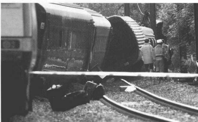
● Figure 1.7 Metal fatigue in the rails is likely to have contributed to the October 2000 Hatfield train crash.
