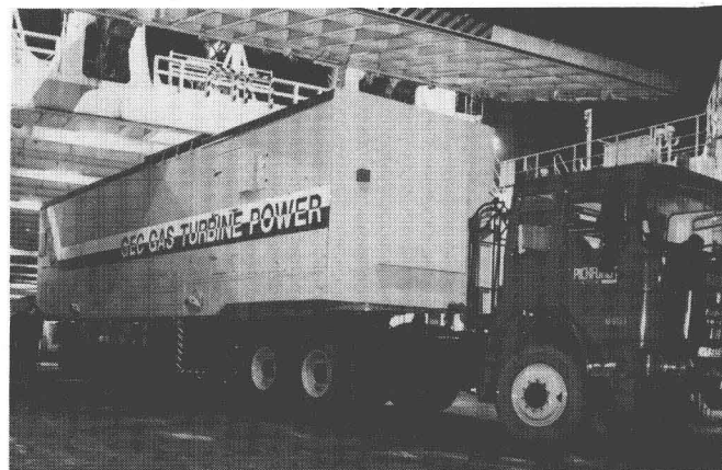
21,600kW Mobile Power Station en route to the Middle East.
