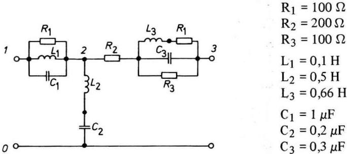
$$\begin{aligned} R_1 &= 100 \, \Omega \\ R_2 &= 200 \, \Omega \\ R_3 &= 100 \, \Omega \\ L_1 &= 0,1 \, \text{H} \\ L_2 &= 0,5 \, \text{H} \\ L_3 &= 0,66 \, \text{H} \\ C_1 &= 1 \, \mu\text{F} \\ C_2 &= 0,2 \, \mu\text{F} \\ C_3 &= 0,3 \, \mu\text{F} \end{aligned}$$
