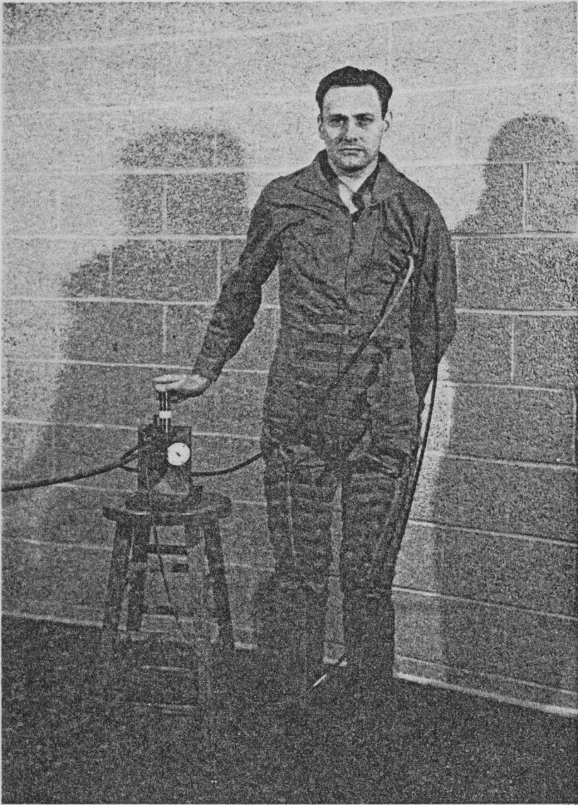
FIG. 11. The David Clark progressive arterial occlusion suit and experimental g valve. Arterial occlusion pressures of about 200 mm of Hg were applied from the ankles upward when the level of +g_z acceleration reached 1.5g and were increased automatically about 52 mm of Hg per g above this level by the g compensated valve, lower left, being activated manually in this picture, 1942. (Reproduced with permission from E. H. Wood et al. , Federation Proceedings 1946, 5, 327.)
