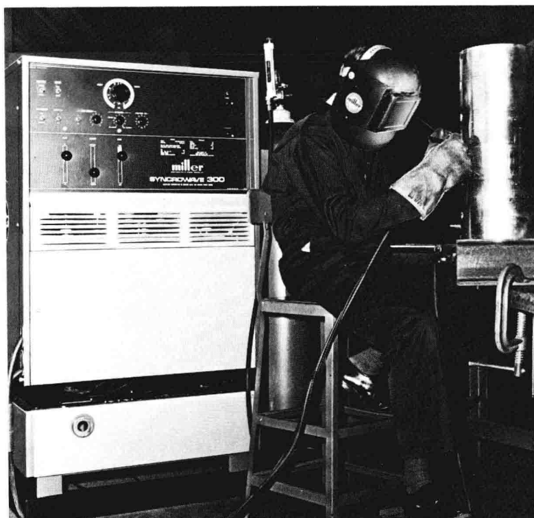
Fig. 2-1. A 300 ampere AC/DC power supply is being used for this manual GTAW operation. Note the helmet, gloves, and dark clothing. (Miller Electric Manufacturing Co.)
