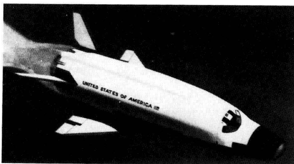
Fig. 6. Single-Stage-To-Orbit (SSTO) Concept that would Take-off Vertically from a Launch Pad and Land on a Runway (Courtesy Rockwell International).
