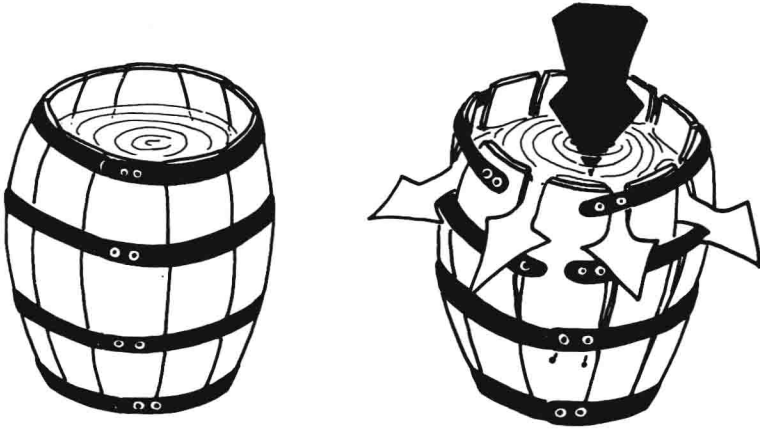
Figure 1.5. Hoop stress. This diagram shows how the load of water in a barrel is resisted by the hoops around the barrel. When too great a load is applied, the hoops will break. The annulus functions in a manner similar to the hoops around a water barrel.
