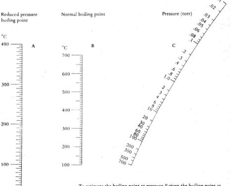
To estimate the boiling point at pressure P given the boiling point at another pressure P': (a) connect pressure P' in C with the boiling point at P' in C using a transparent ruler and insert a needle or sharp pin at the point where the ruler intersects line C; (b) pivot the ruler around the needle until it reaches the desired pressure C in C, then read the boiling point at C from C.
