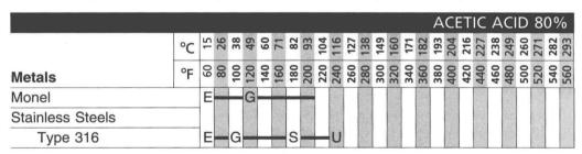
From the sample table, it is seen that in the presence of an 80% solution of acetic acid, monel has a corrosion rate varying with temperature rated as follows:
