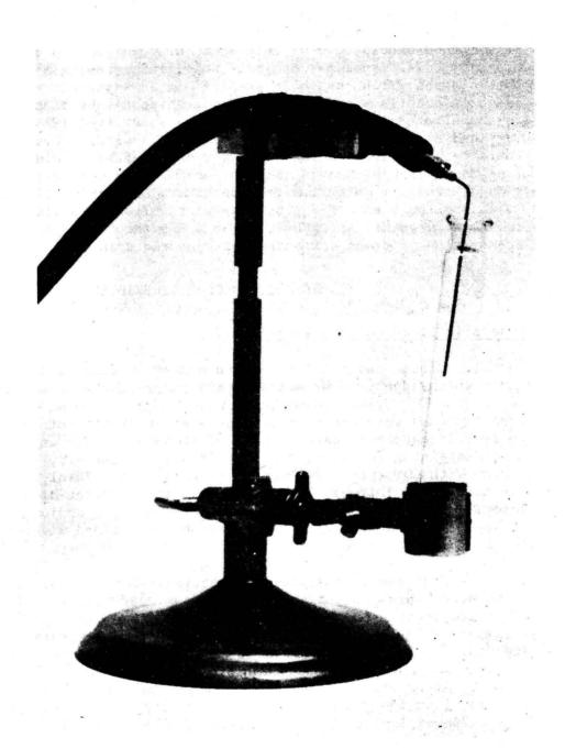
Figure 2. The "open" method of collection consists of removing the stopper from a sterile tube and placing a cannula in the tube so that a continuous flow of oxygen-free gas may be used to prevent ingress of air.
