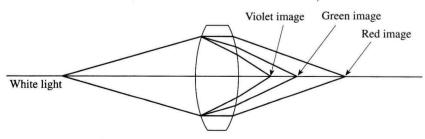
FIGURE 1-6 Schematic illustration of chromatic aberration.
