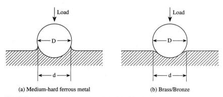
FIGURE I-I Schematic illustration of the Brinell hardness test.
