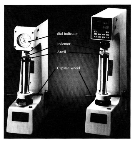
FIGURE I-2 A photograph of a Rockwell hardness testing apparatus. (Courtesy of Buehler Ltd.)
