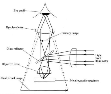
FIGURE 1-4 Schematic illustration of the metallurgical microscope.
