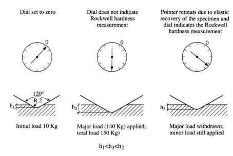
FIGURE 1-3 The procedure for performing a Rockwell hardness test (on the C scale).
