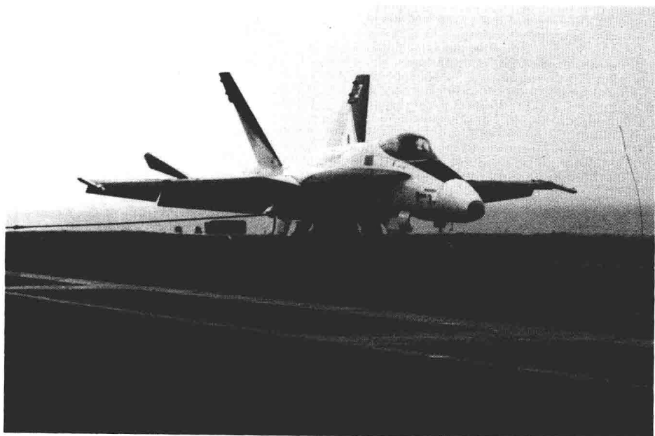
The main landing gear of a Hornet abruptly changes its appearance as the plane settles onto a carrier deck. The gear bends at the "knees" and seems to crouch beneath the plane. ( McDonnell Douglas Co. )
