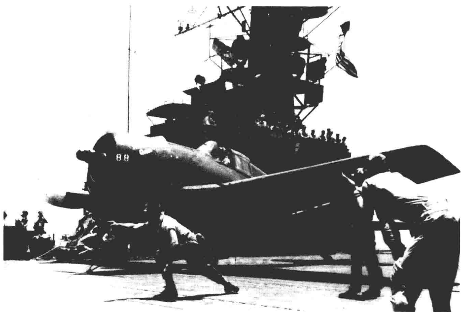
A Grumman F-6F-5N Hellcat of VMF-511 gets the signal for takeoff near Okinawa in May 1945. Note the radar antenna protruding from the right wing. Installed late in the war, radar permitted the Hellcat to operate as a night fighter. ( Smithsonian Institution. )
