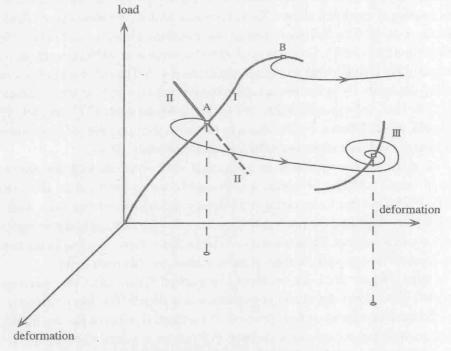
FIG. 1. Initial stable response followed by collapse.
