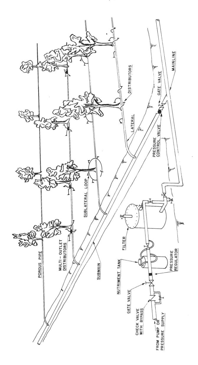
Basic components of a localized irrigation system
