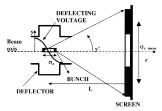
Figure 1. Longitudinal to transverse correlation induced by the RFD transverse voltage.
