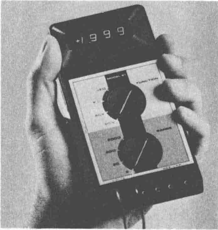
Fig. 1-6. A portable digital multimeter with LED (light emitting diode) readouts. It is used to troubleshoot electronic instruments. (Data Technology Corp. / Santa Ana, Calif.)
