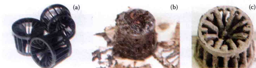
FIGURE 13.11 Photographs of biological solids attached to the anaerobic fixed bed media. (a) Noncolonized support, (b) colonized support, and (c) support after heat drying.
