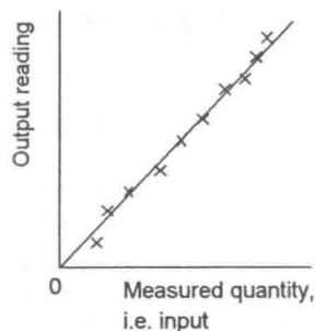
Figure 1.19 Sensitivity as slope of input-output graph
