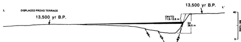
FIGURE 2. Example of slip rate calculation for a normal fault. The displaced datum is a 13,500-year-old terrace surface displaced by the Wasatch fault. The stippled band is the projection of the surface across the fault zone. The fault scarp at this location is 28.5 m high but the cumulative net vertical tectonic displacement (CNVTD), which is the displacement used for the slip rate, is 11.5–13.5 m. This yields a slip rate of 0.85–1.0 mm/yr. for the past 13,500 years. Similar types of measurement can be made for strike-slip and reverse faults. Vertical scale = horizontal scale. (Modified from Swan et al. , 1980).
