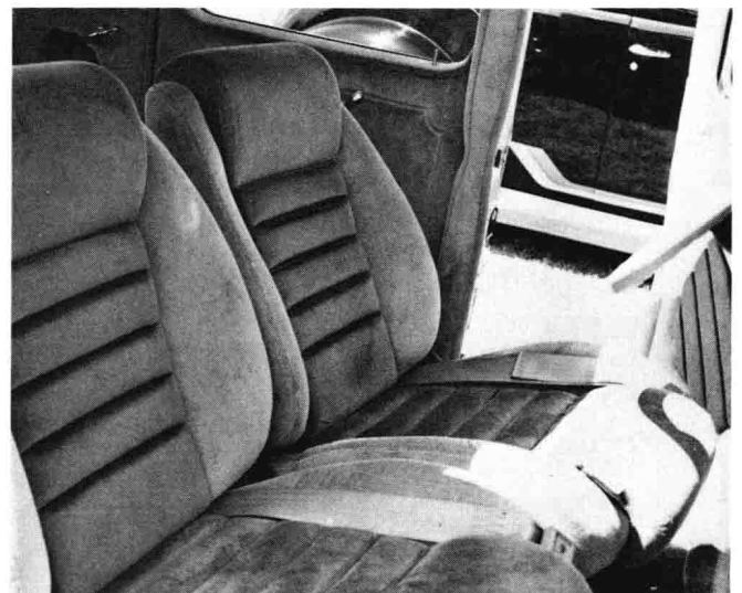
Front bucket seats offer comfort in this four-door street rod. Modern body-support styling and tan velour material similar to the original mohair are featured in this Model A.
