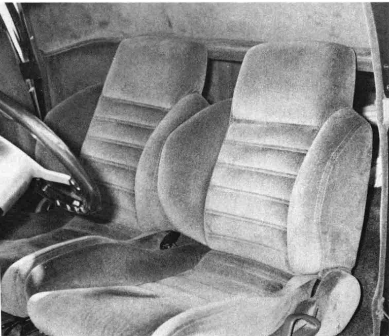
Form-fitting, competition-style seats give a car a performance feel. These seats were specially built. Several designs are available from various suppliers in finished or unfinished form.
