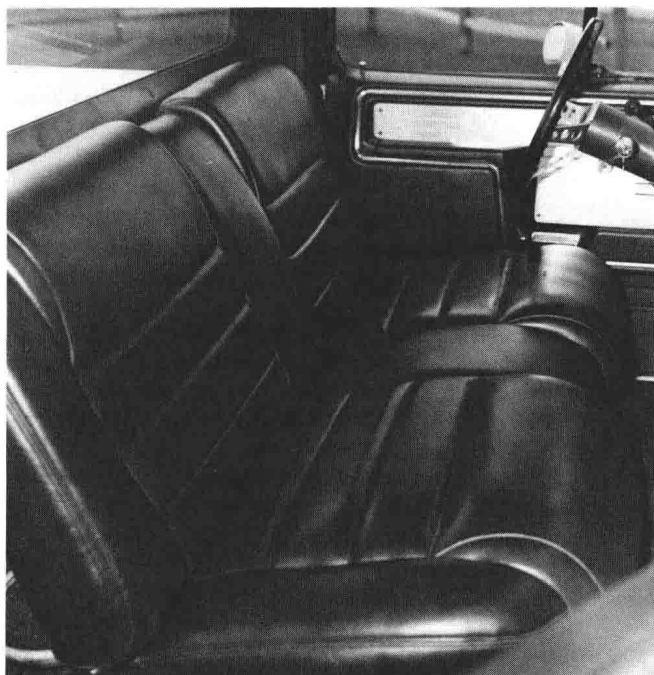
A solid bench seat used in a pickup, early coupe or roadster. Dale Boesch chose a black vinyl bench for his 1980 Forst pickup with wide, horizontal rolls and extra padding in the shoulder and leg support areas.
