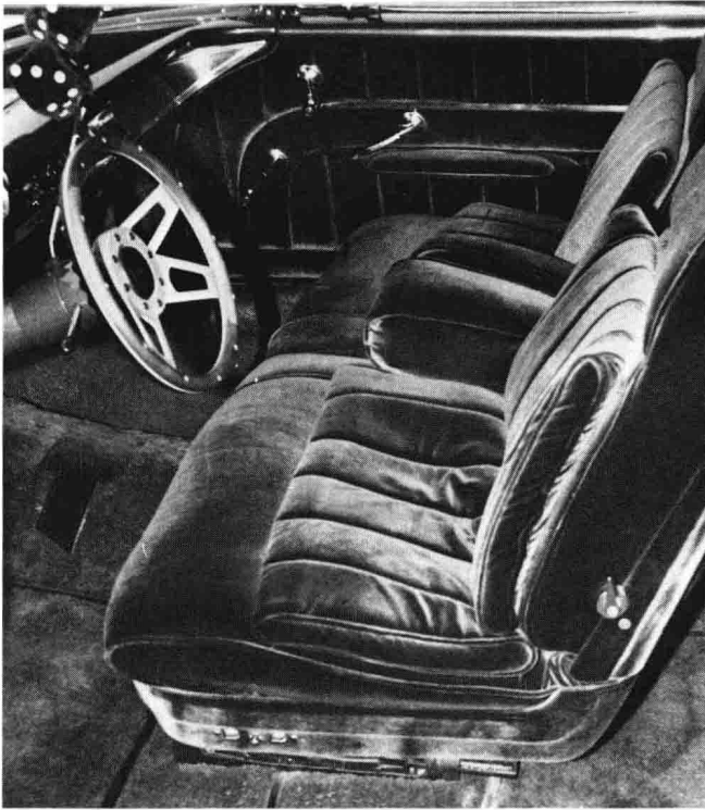
The plush padding and fabrics of a late-model luxury car appear in this contemporary interior. Dan and Sharon Botos transplanted dark brown velour power seats from a 1983 Lincoln Town Car into their 1957 Chevy.
