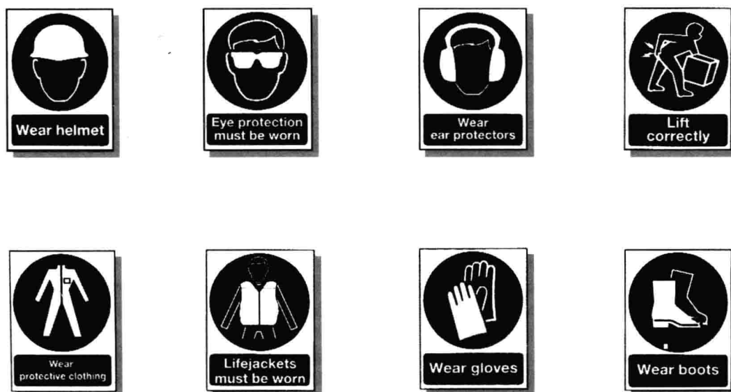
Fig. 1.2 Safety signs showing type of PPE to be worn.
