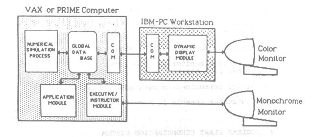
Fig. 1: Compact Analyzer Software Design
