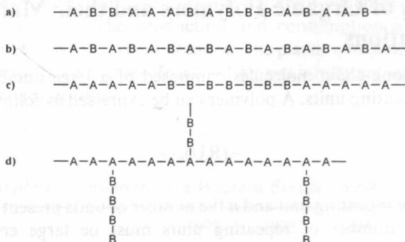
Figure 1.3 Possible structures of copolymers containing A and B repeating units: (a) random, (b) alternating, (c) block, (d) graft.
