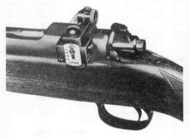
Lyman No. 57 Receiver Sight. Each graduation on the slide is 3 minutes. Turning the coin-slotted head one complete revolution elevates the sight 3 minutes, or turning it one graduation elevates a quarter minute. One minute changes the point of impact one inch per hundred yards. Windage works similarly. Redfield No. 70 Receiver Sights work on the same principle. Note the cup disc which should always be unscrewed for hunting.
