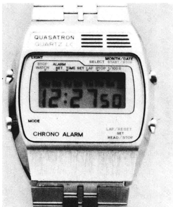
A quartz-crystal regulated wristwatch. The digital read-out is a liquid crystal display (LCD).
