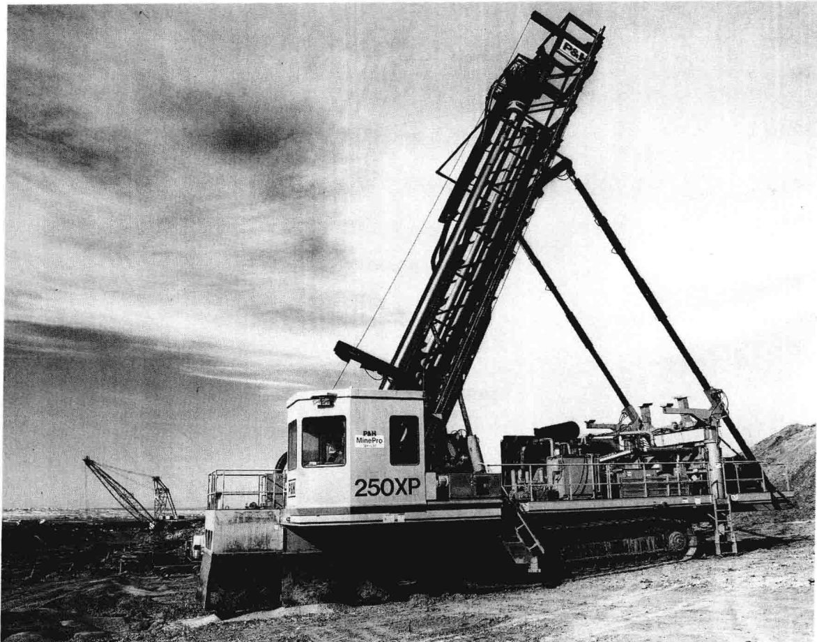
Figure 1.2 A hydraulically operated rock drill. (Courtesy of P&H Mining Equipment)
