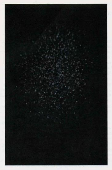
**FIGURE 0.1**Random interference pattern generated when laser light is scattered by ground glass. (See color insert following page 14.)
