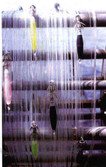
6. Soft body and hard body (black) squid jigging hooks on reel – Japan (C.F.E. Roper)
