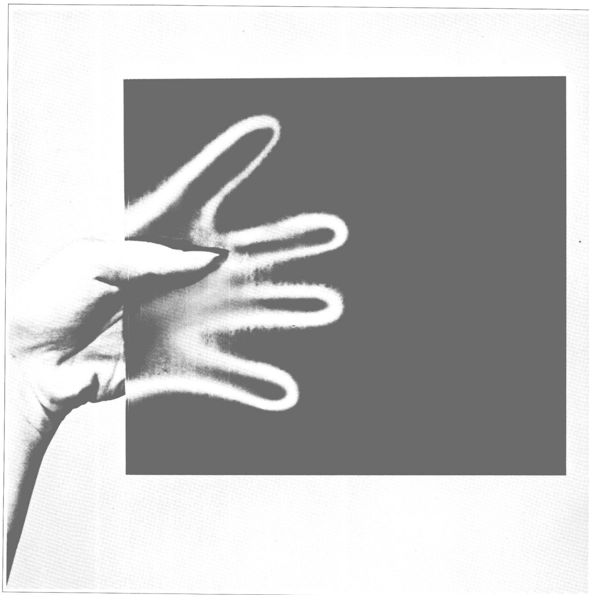
Liquid crystals on a sheet of plastic. The color of the crystals is related to their temperature. (Courtesy LiquiCrystal, Inc., York, Pennsylvania)
