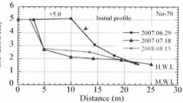
Figure-6 Embankment profile (No.-70)
