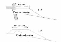
Figure-5 Profiles of nourished embankment
