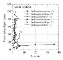
Figure-9 N-value on the crown of nourished embankment on South section
