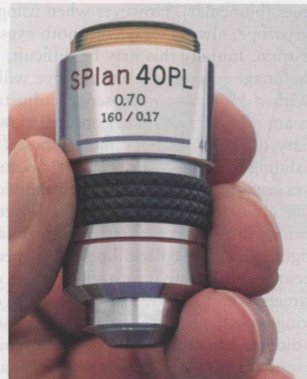
FIGURE 1-6 Engravings on this objective indicate that it is a planachromat lens (SPlan); the initial magnification is 40×; the numerical aperture is 0.70; the objective is designed for a microscope with an optical tube length of 160 mm; and the coverslip thickness should be 0.17 \pm 0.01 mm.
