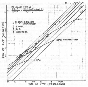
FIG. 1—Relationship between penetration at 25°C (77°F), penetration at  $10^{\circ}$ C (50°F) PI, and cracking temperature for bitumens (after Ref 5).
