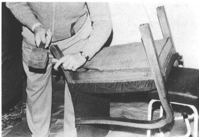
6. Removing tacks in direction of timber grain
