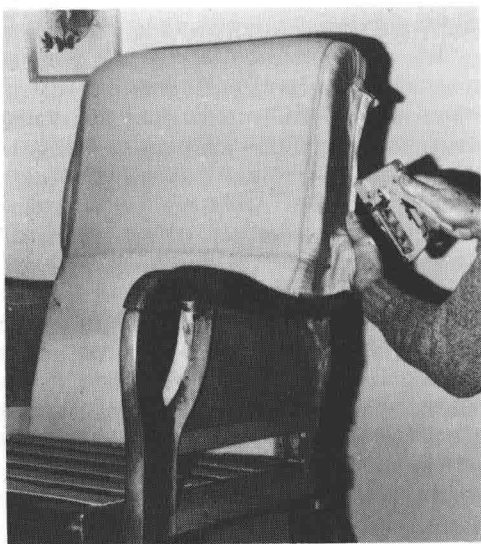
2. Using hand stapling tool
