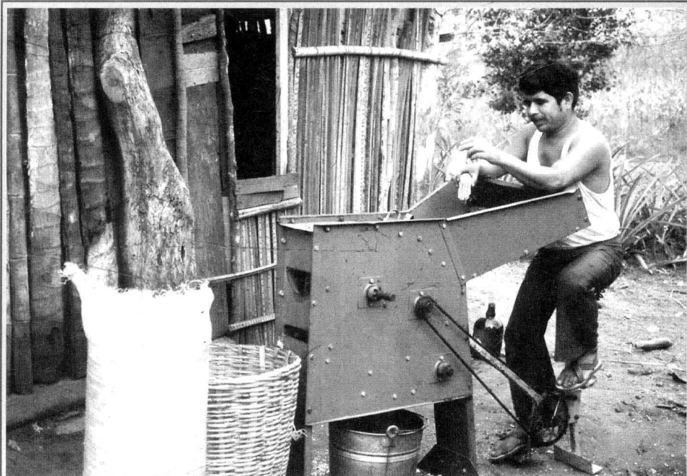
FIGURE 4 Shelling maize by using a machine considerably reduces drudgery and time. (Photo by B. Sims)
