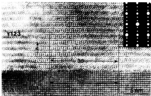
Figure 1.1. HRTEM image of the interface between the YBCO film deposited by PLD and the LaAlO 3 (001) substrate. The inset SAED pattern taken from an area including both the film and the substrate confirms the epitaxial growth. The presence of an interfacial dislocation is seen in form of an extra half-plane in the substrate within the marked regions. From [14].
