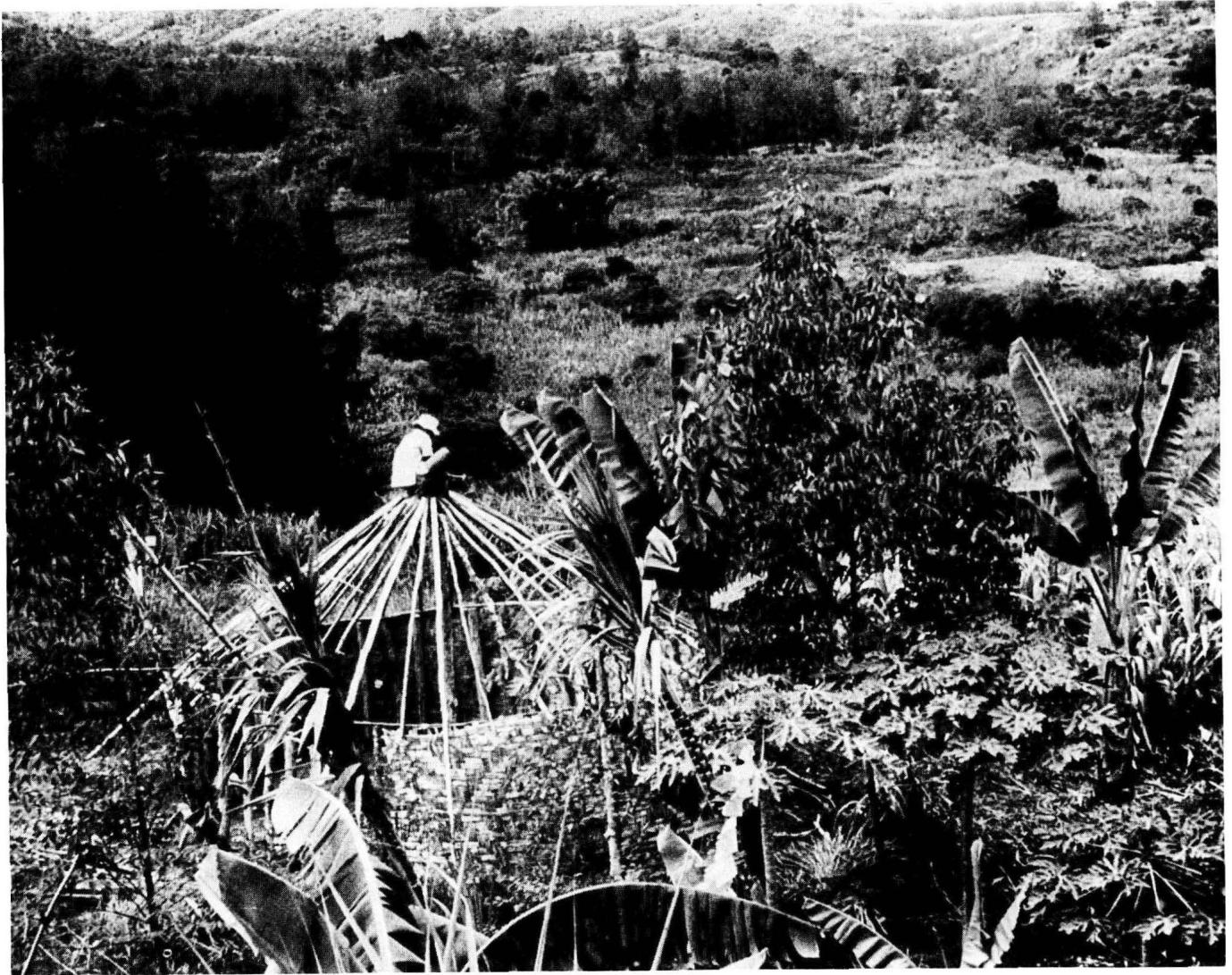
Fig. 1.1.3. Circular hut in the Highlands of New Guinea, made of bamboo tied together with vegetable fibers. The walls are woven mats and the roof is thatch. The hut can be erected by two people in a single day, if they have previously collected the materials from the surrounding countryside, cut the poles to length, and woven the mats.
