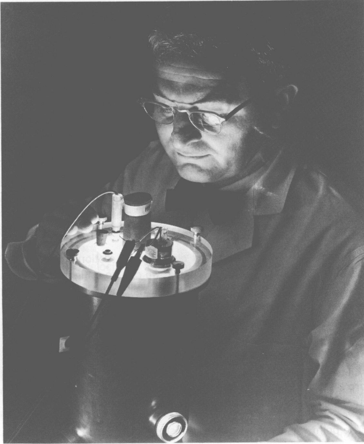
Figure 1.1 A National Bureau of Standards scientist adjusts a krypton-86 lamp in its liquid nitrogen bath. The wavelength of the orange-red light emitted by the lamp has been adopted as the international standard of length. (Courtesy of the National Bureau of Standards, Washington, D.C.)
